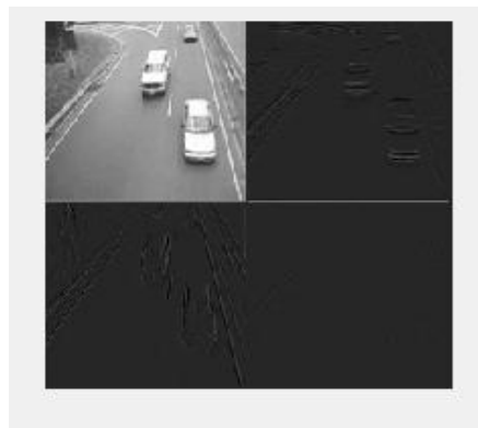
Fig.7. Corner Detection with noise removal
